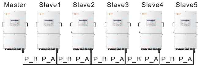
Figure 3.23 Parallel Terminal Connection
