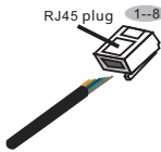
Figure 3.23 Strip the insulation layer and connect to RJ45 plug
